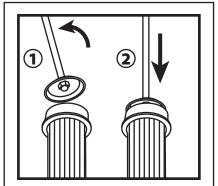
**DIAGRAM A:** For ease of use put the piston into the barrel at a slight angle (1) and then straighten the rod and push in (2).
