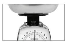
Adjust the pointer to zero by turning the knob which is located under the tray on the front of the scale.
