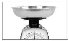
3. Tap the pan gently to settle the mechanism. If necessary, re-adjust each time you use the scale.
