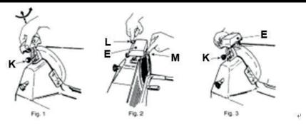
Should the Blade become dull it will be necessary to sharpen it. This slicer comes equipped with built-in sharpener.
