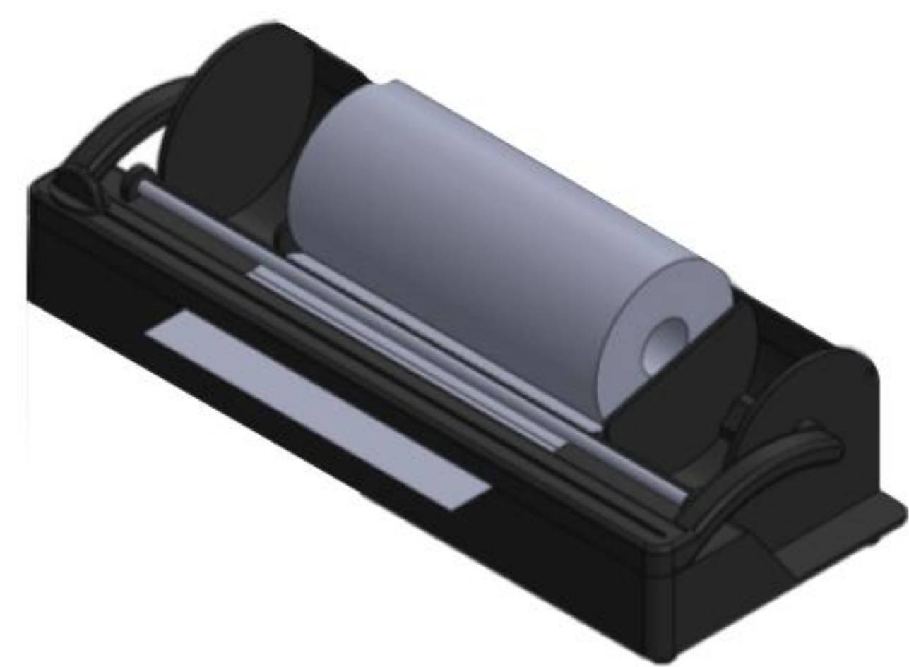
Feed material under the fixed rod and cutting bar.
